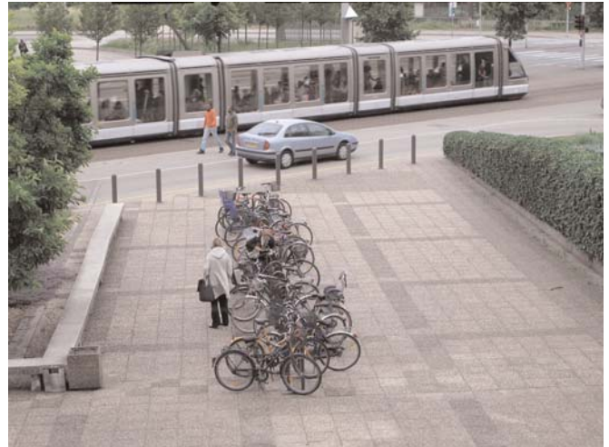
Figure 3 Strasbourg's trams were designed to have very large windows to provide passengers with a wide view of the city and to have low floors, ensuring easy access for passengers with disabilities and passengers pushing strollers or carts.
